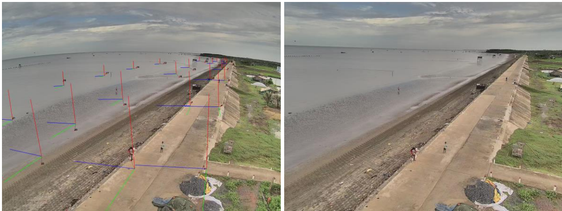
Figure 9: Camera image calibration and rectification. Original (left) and corrected images (right): the horizon line forms a circle arc in the original image and a straight line on the corrected image. On the original image, all ground control points are shown with their respective projection in pixel space. A 3-axe reference frame is drawn on each point to check consistency of geographical reference system.
