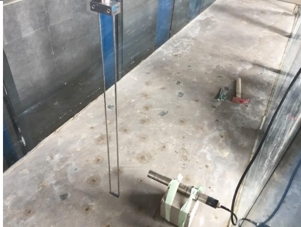
Figure 3-15 Placement of wave gauges and turbidity sensors
