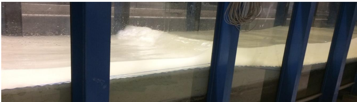
Figure 3-30 Severe wave breaking at the sandbank outer slope
