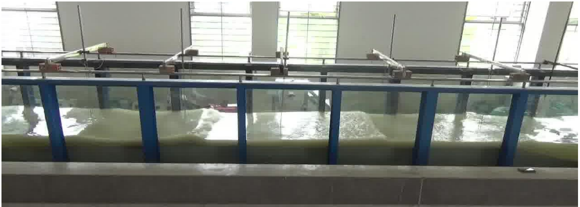
(c) Sandbank deformation after testing
