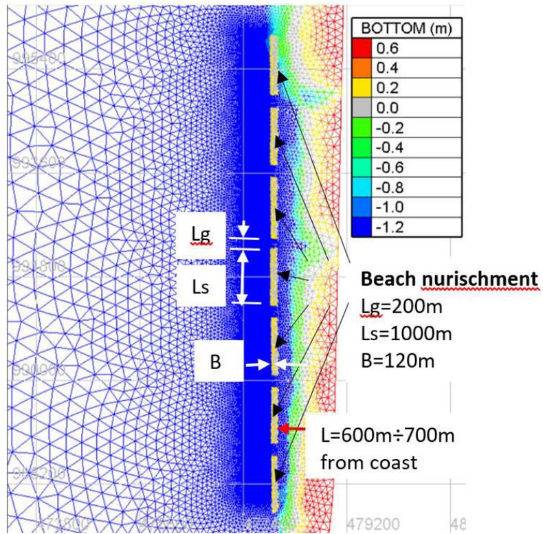
Figure 2.1d: Simulation of nourishment interrupted bed in study area
