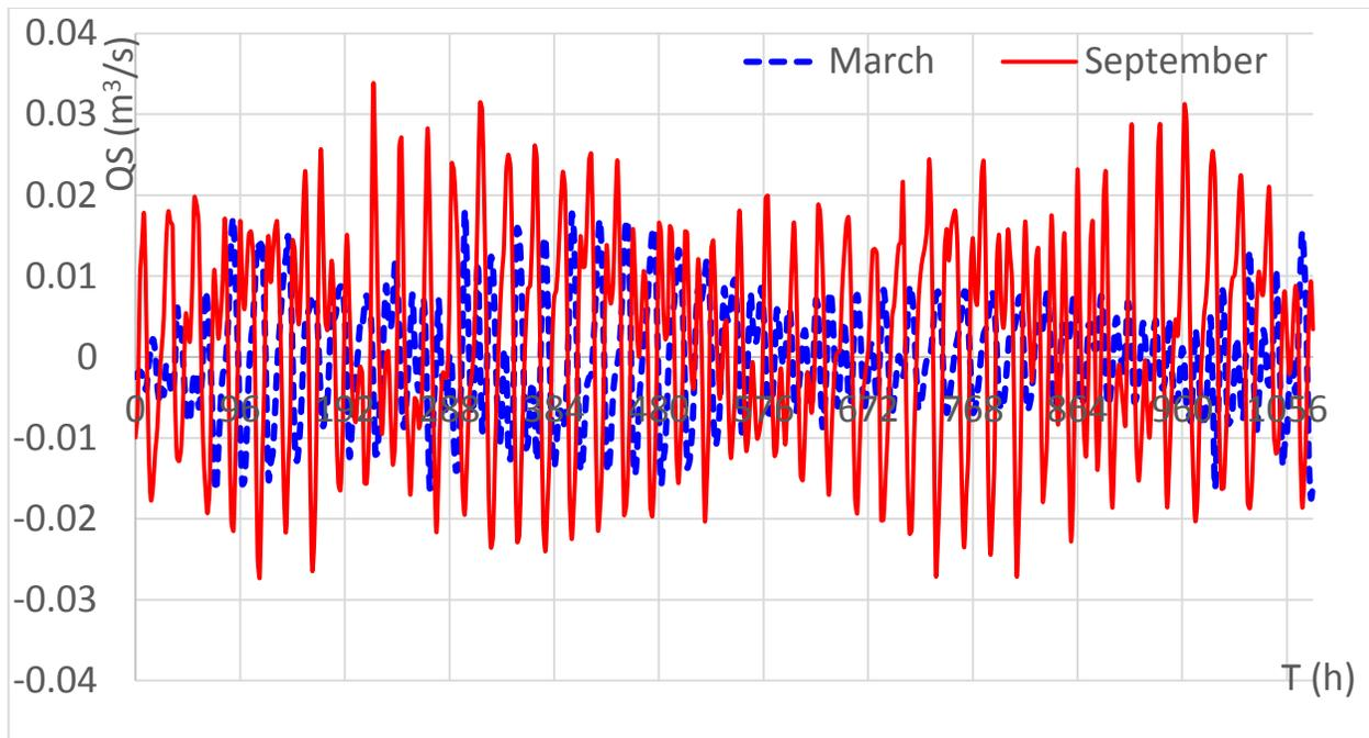
Figure 3.5: Sediment fluxes through cross section 1-1 over time in case with beach nourishment.
