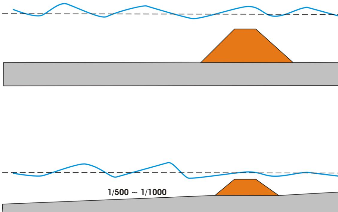
Figure 1.1: Typical type of beach nourishment for wave attenuation
