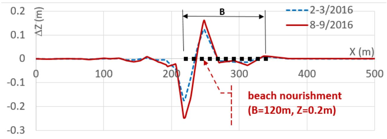
Figure 3.3: Accumulated evolution of bathymetry at section 1-1 in case with beach nourishment (B=120m, Z=0.2m). The continuous line stands for 8-9/2016 and the dashed line stands for 2-3/2016.
