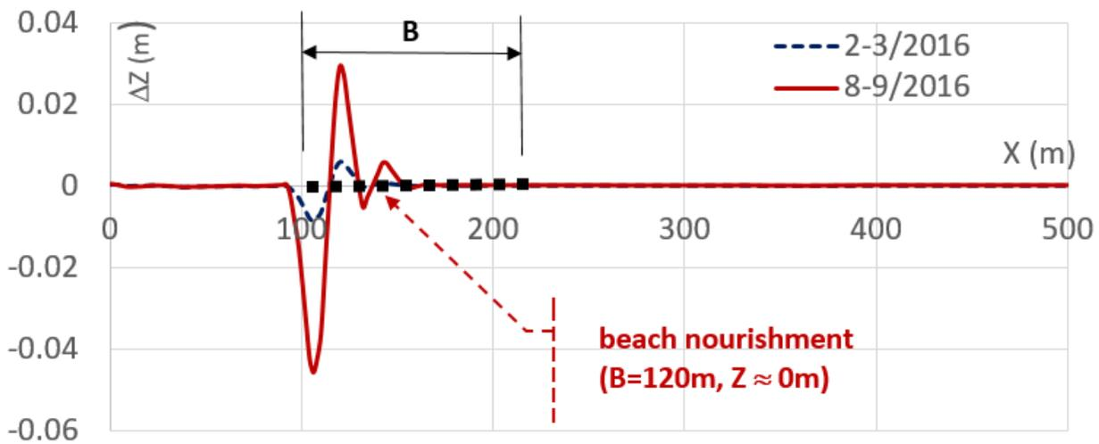
Figure 3.4: Accumulated evolution of bathymetry at section 1-1 in case with beach nourishment ( $B=120$ m,  $Z=0$ m). The continuous line stands for 8-9/2016 and the dashed line stands for 2-3/2016.
