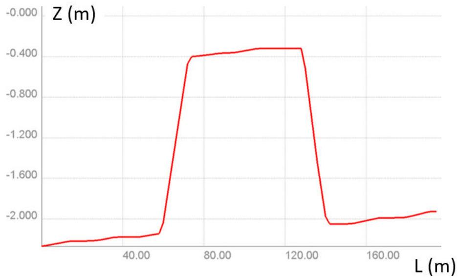
Figure 2.1c: Cross-section A-A, dimension of BN is B=60m in width and H=1.7m height
