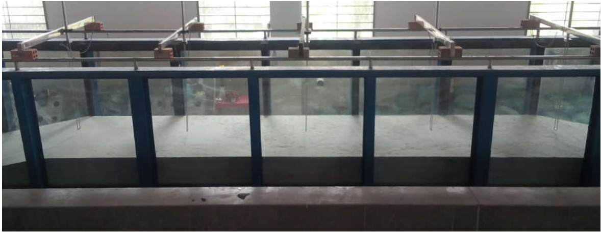
(b) During testing: severe wave breaking and high sediment concentration
