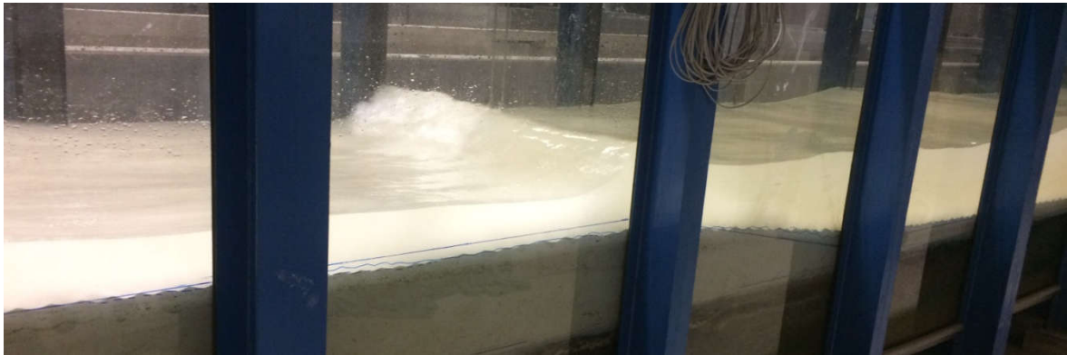
Figure 19 Severe wave breaking at the sandbank outer slope
