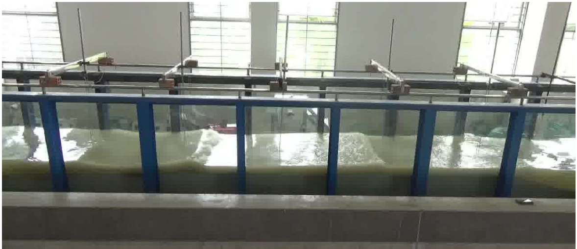
(c) Sandbank deformation after testing
