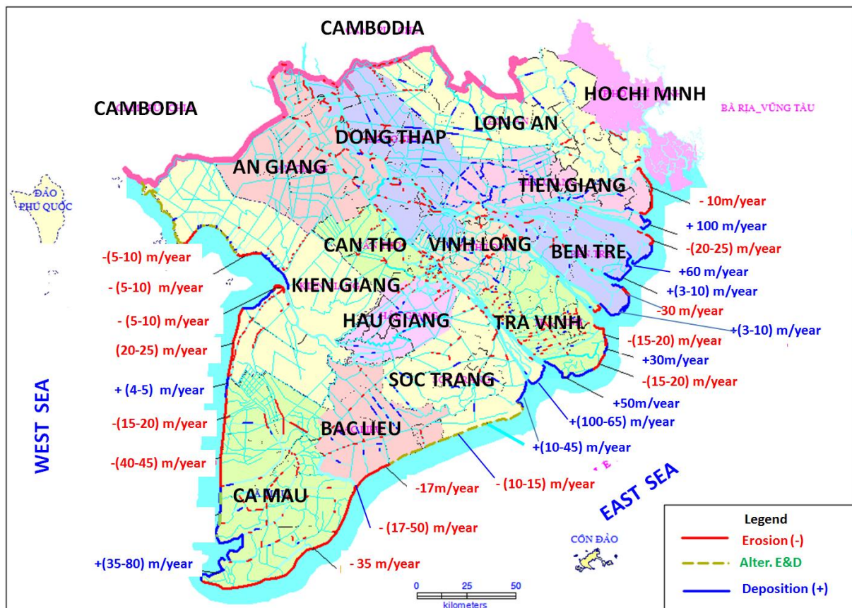
Figure 2. Existing erosion and deposition situation along the coastline of LMD
